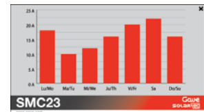
Week graphic Displays columns with day average aggregate during last 7 days.
